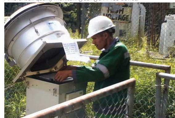
Ambient air quality monitoring using a PM 10 device.
