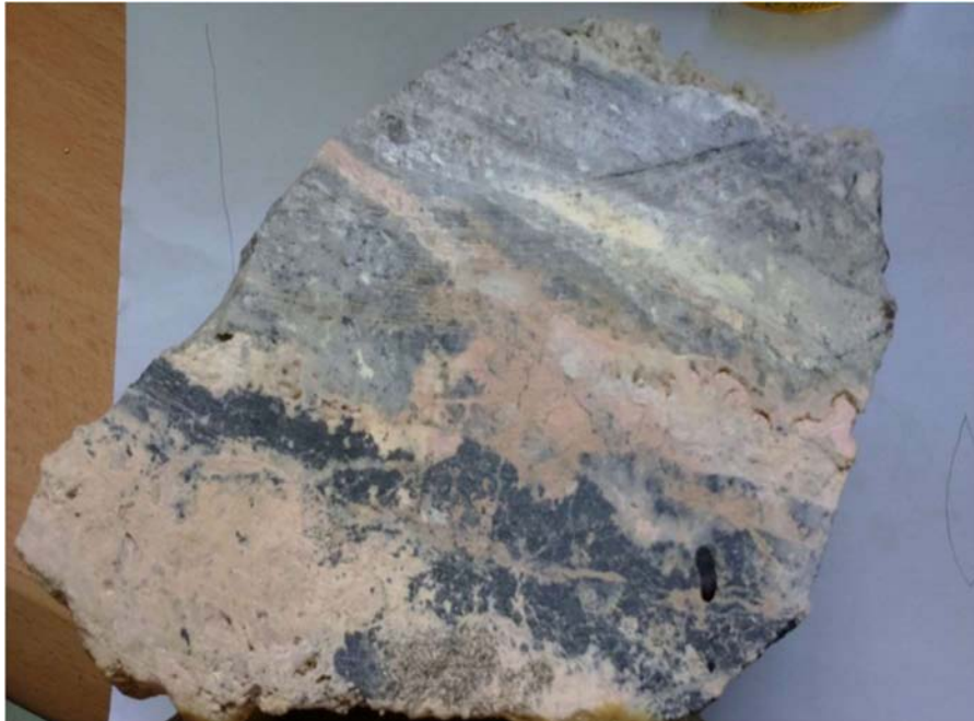
Figure 13-14: Level 590 SDNS ODW hand specimen showing quartz-carbonate-galena crustiform-colloform bands. Incorporated silicified diorite clasts with relict feldspar laths and disseminated cpy-py.
