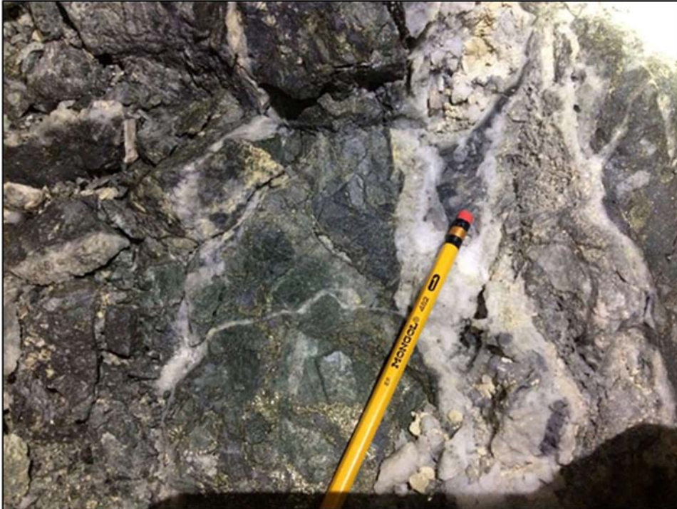
Figure 13-10: Carbonate+quartz vein breccia with py+cpy disseminations and patches exposed underground at heading Level 560 SDNS ODE 102S position
