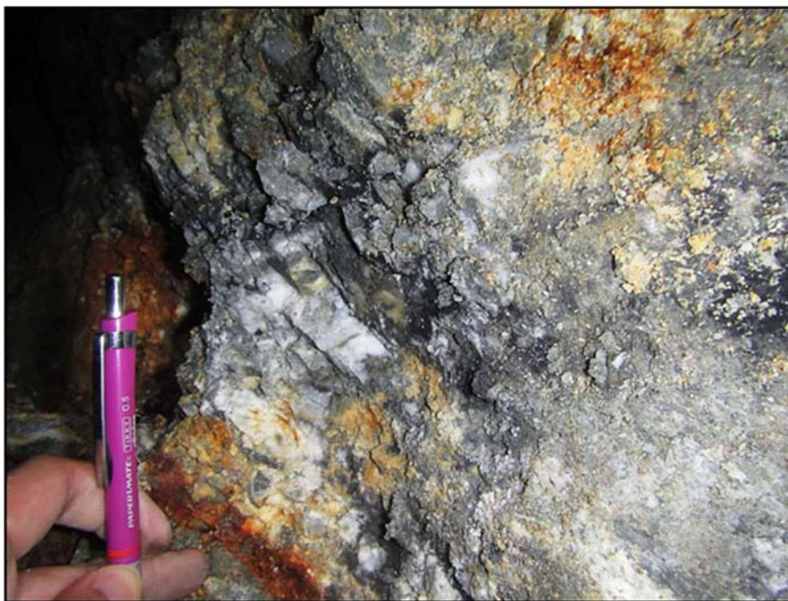
Figure 13-13: Grey and white chalcedonic quartz veins associated with black sulfide veinlets exposed at Level 545 MST2 ODW 52N position
