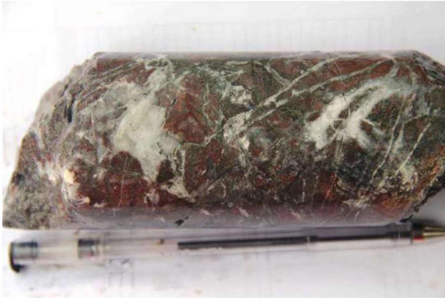
Figure 13-17: Monomictic crackle breccia characterized by angular garnet skarn clasts set in vuggy, drussy quartz+calcite vein intercepted in DNC-530-104 at 85.4m
