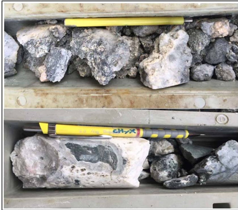
Figure 13-7: Quartz-carbonate vein breccia intercept in MST-560-004 at 117.4-117.7m. Carbonate veins show colloform-crustiform banding
