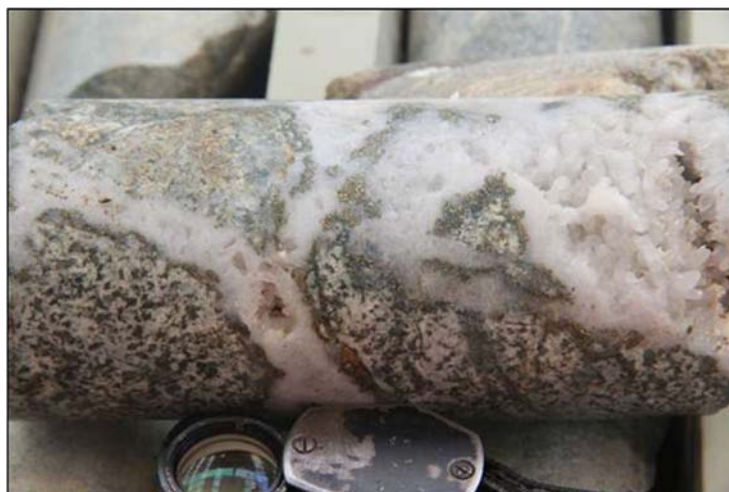
Figure 13-9: Vuggy quartz+pyrite+chalcopyrite vein with angular diorite clasts in ASA-590-020 at 56.8-57.8m. Sulfides occur along vein selvages.
