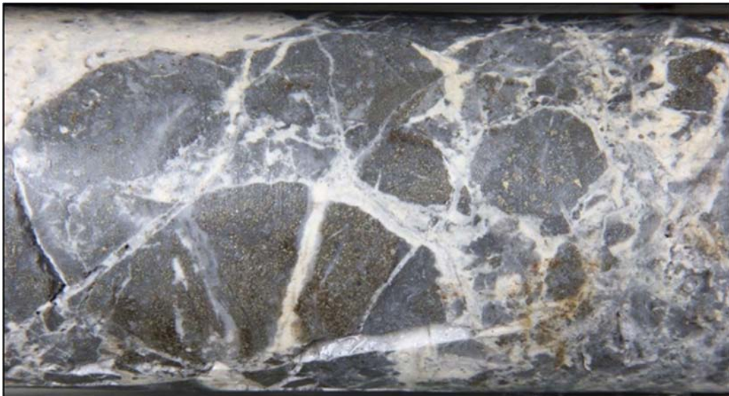
Figure 13-5: ASA-590-004 intercept displaying multi-phased breccia with angular to sub-angular sulfide-rich clasts and quartz-calcite-rhodochrosite veins
