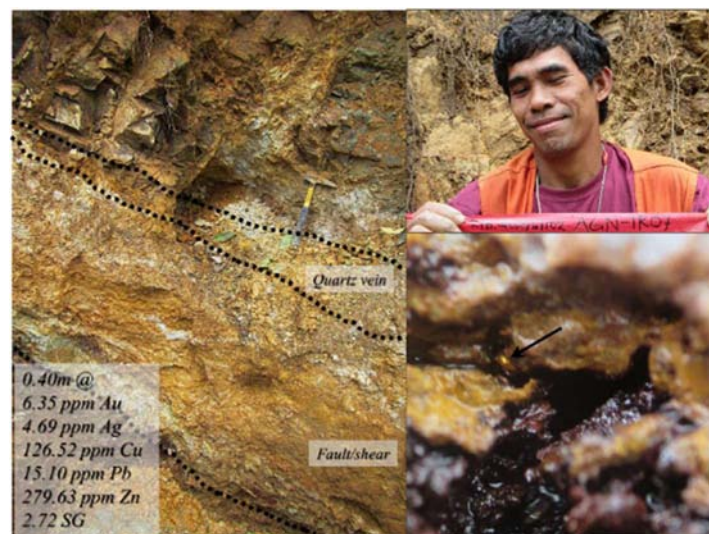
Figure 14-8: Quartz vein further exposed via trenching. Lower right picture pointed by arrow shows liberated gold
