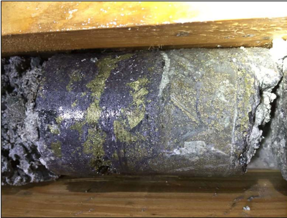
Figure 13-5: (Cover Photo) Massive sulfide (gn+py+cpy) vein breccia intercept in MST-590-008
