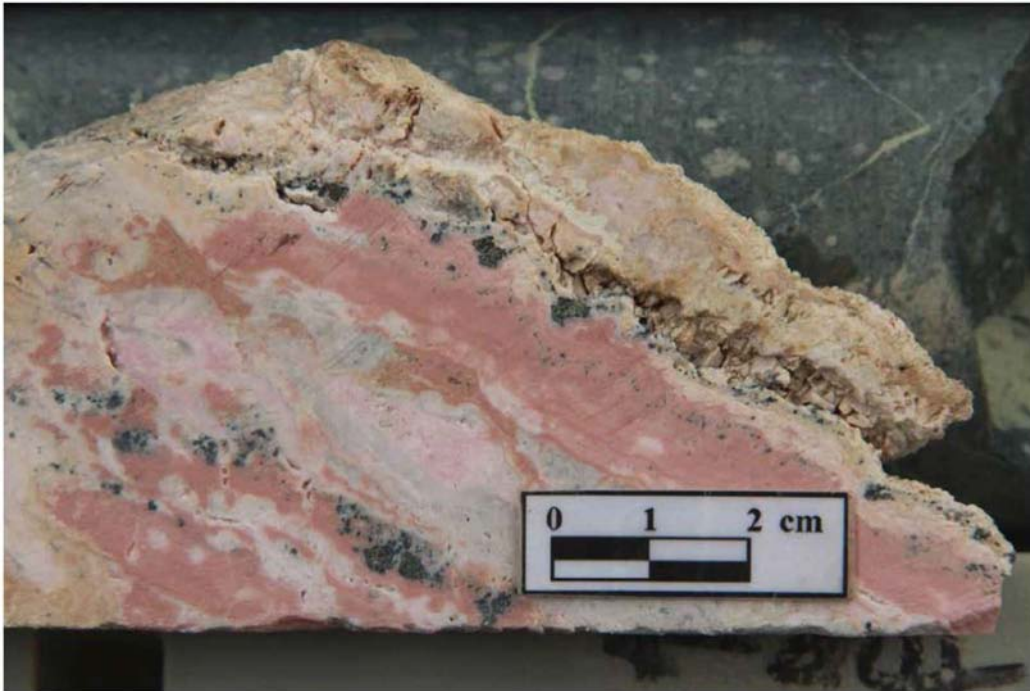
Figure 13-4: ASA-785-012 intercept at 330.7m showing crustiform-colloform banded quartz+rhodonite+rhodochrosite+sulfide vein and late stage vuggy carbonate veins with bladed texture
