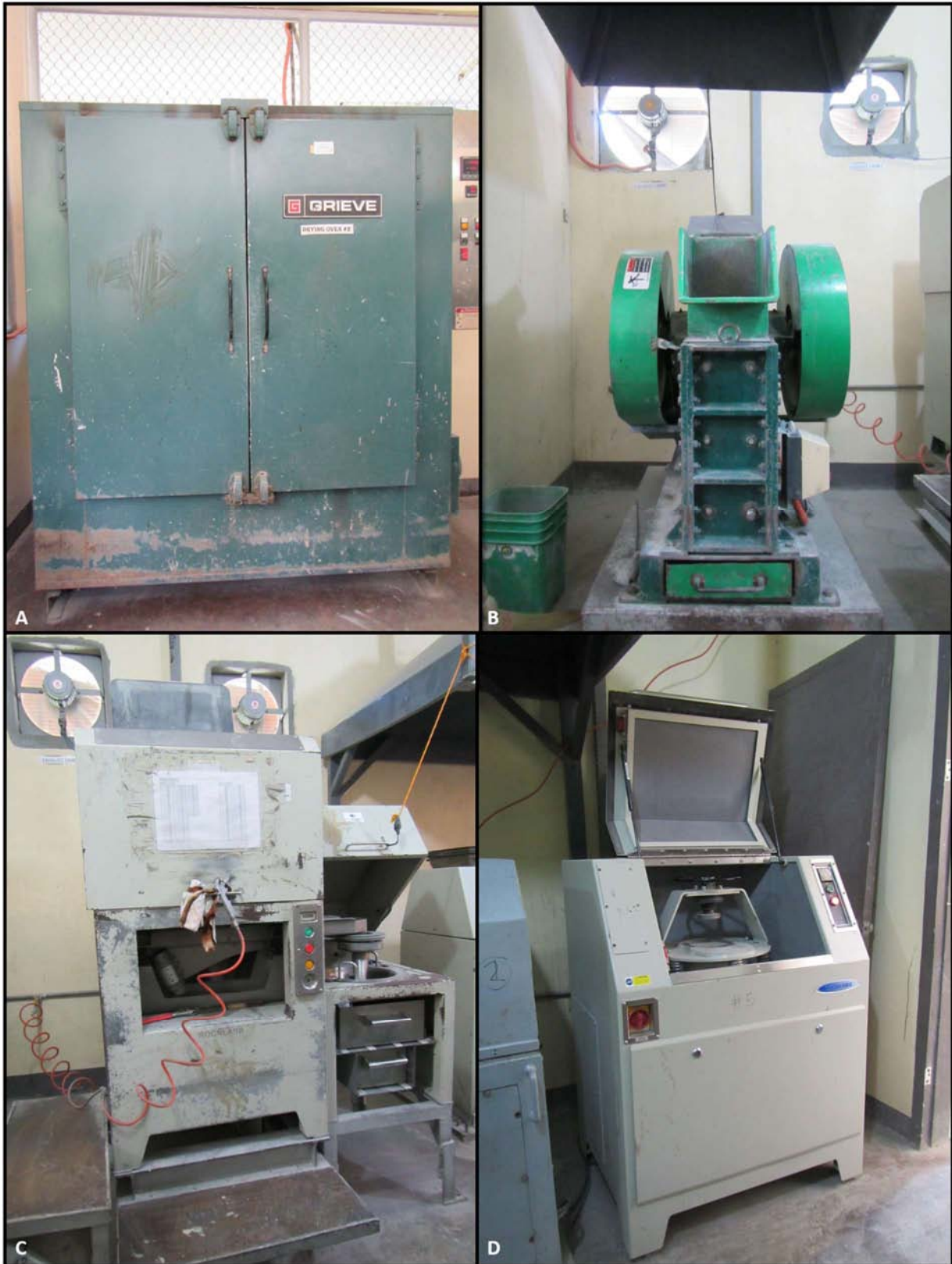
Figure 15-3: Sample Preparation Equipment: (A) Drying Oven (B) Jaw Crusher (C) Boyd Crusher (D) Pulverizer
