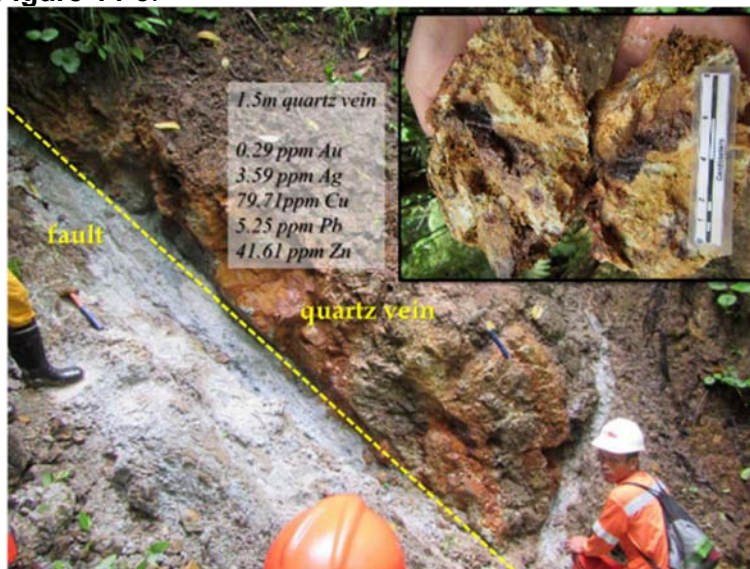
Figure 14-3: Kaurangan trench no. 21 with quartz vein and associated fault. Inset shows quartz vein breccia hand specimen
