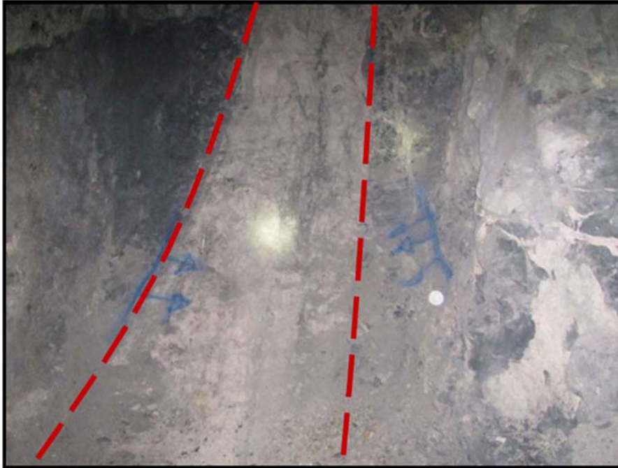
Figure 13-19: Approximately 1.2m wide carbonate+base metal sulfide vein exposed at Level 590 SDN ODE MV 134S position. The vein is composed of carbonates, galena-sphalerite stringers/lenses with minor rhodochrosite and disseminated py+cpy
