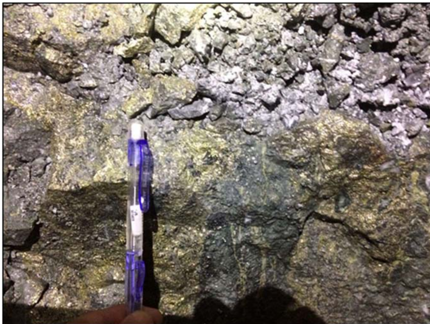
Figure 13-11: High Au grade massive sulfide (py-cpy) vein hosted by propylitic-altered andesite at Level 490 BNZ ODE
