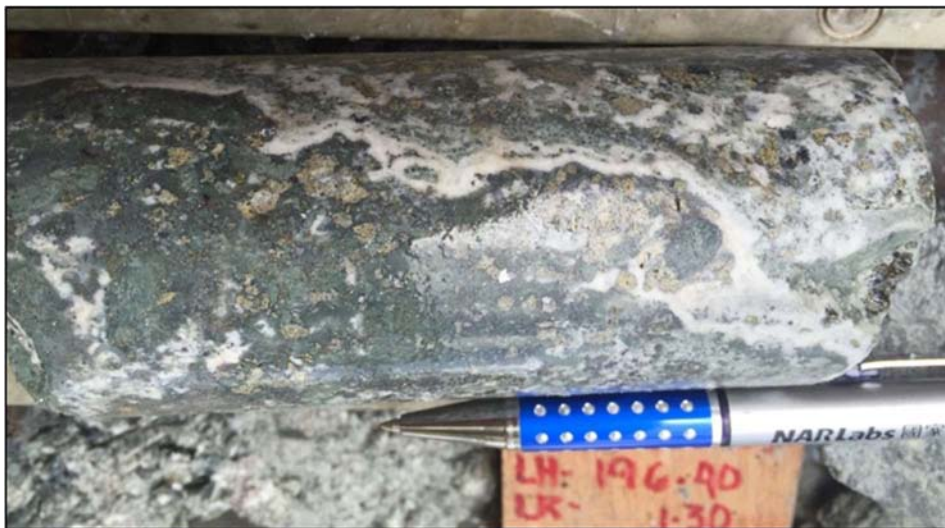
Figure 13-3: MST-590-005 intercept at 194.1-195.1m interpreted as part of the Don Calixto vein characterized by multiphase base metal-carbonate mineralization
