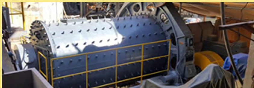
9'x15' Allis Chalmers ball mill for the Sangilo Mine
