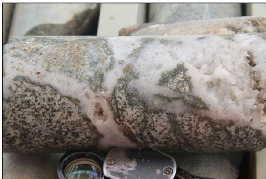
13.1.1.8. Vuggy quartz+pyrite+chalcopryite vein with angular diorite clasts in ASA-590-020 at 56.8-57.8m. Sulfides occur along vein selvages.
