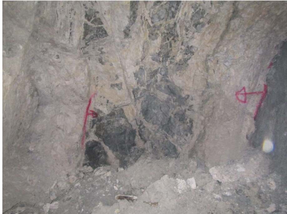
13.3.3 Multiphase vein zone exposed at Level 756 SDY ODE 142S position. The 3.5m wide vein zone is composed of sulfide-quartz breccia with late carbonates. Sulfides are comprised primarily of pyrite and chalcopyrite with minor galena and sphalerite.
