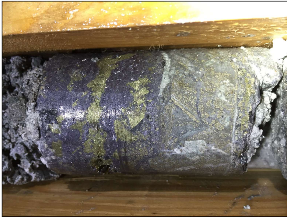
13.1.1.3. ASA-590-004 intercept displaying multi-phased breccia with angular to sub-angular sulfide-rich clasts and quartz-calcite-rhodochrosite veins.
