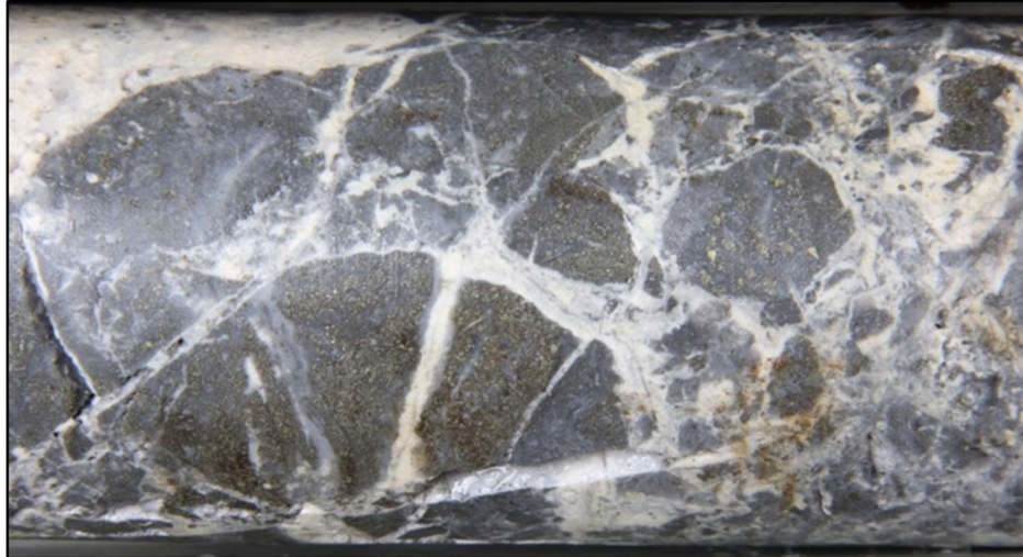
13.1.1.3. ASA-590-004 intercept displaying multi-phased breccia with angular to sub-angular sulfide-rich clasts and quartz-calcite-rhodochrosite veins.
