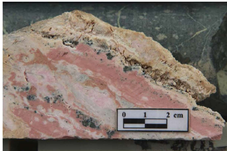
Figure 13-2. MST-590-005 intercept at 194.1-195.1m identified as Don Calixto vein and characterized as base metal - carbonate vein.
