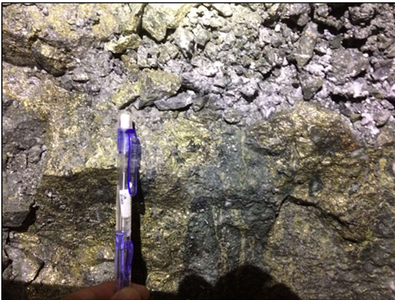
13.1.1.10. High Au grade massive sulfide (py-cpy) vein hosted by propylitic-altered andesite at Level 490 BNZ ODE.
