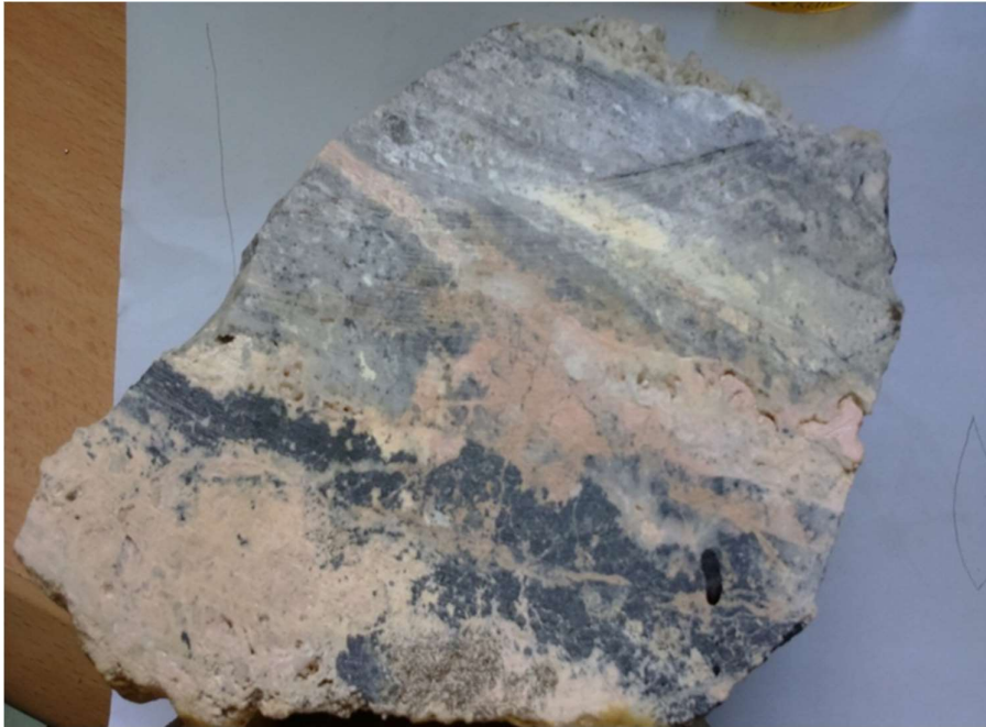
13.1.1.13. Level 590 SDNS ODW hand specimen showing quartz-carbonate-galena crustiform-colloform bands. Incorporated silicified diorite clasts with relict feldspar laths and disseminated cpy-py.
