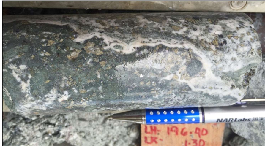
Figure 13-2. MST-590-005 intercept at 194.1-195.1m identified as Don Calixto vein and characterized as base metal - carbonate vein.
