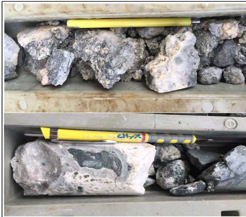
13.1.1.6. Quartz-carbonate vein breccia intercept in MST-560-004 at 117.4-117.7m. Carbonate veins show colloform-crustiform banding.
