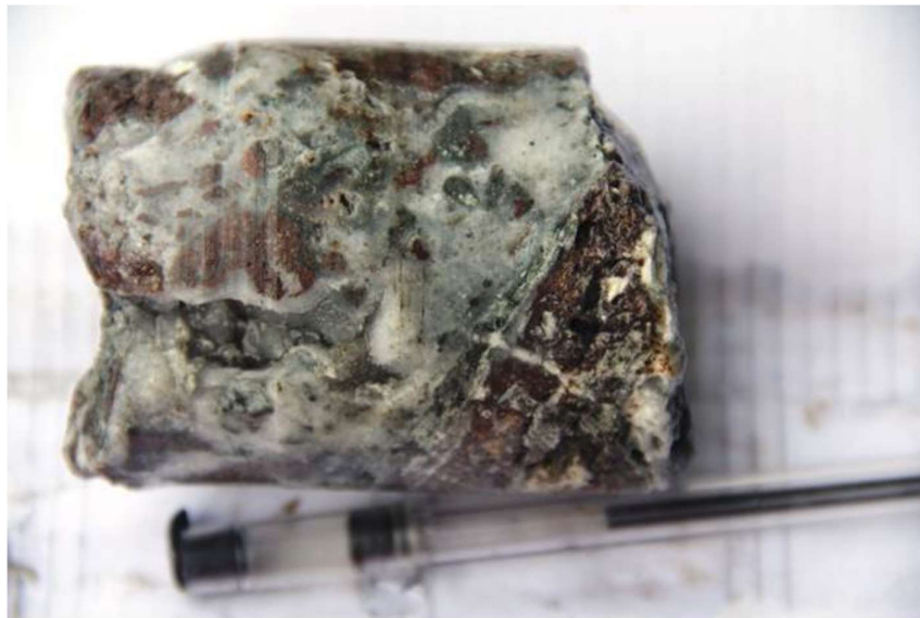
13.1.3.2. Monomictic crackle breccia characterized by angular garnet skarn clasts set in vuggy, drussy quartz+calcite vein intercepted in DNC-530-104 at 85.4m.
