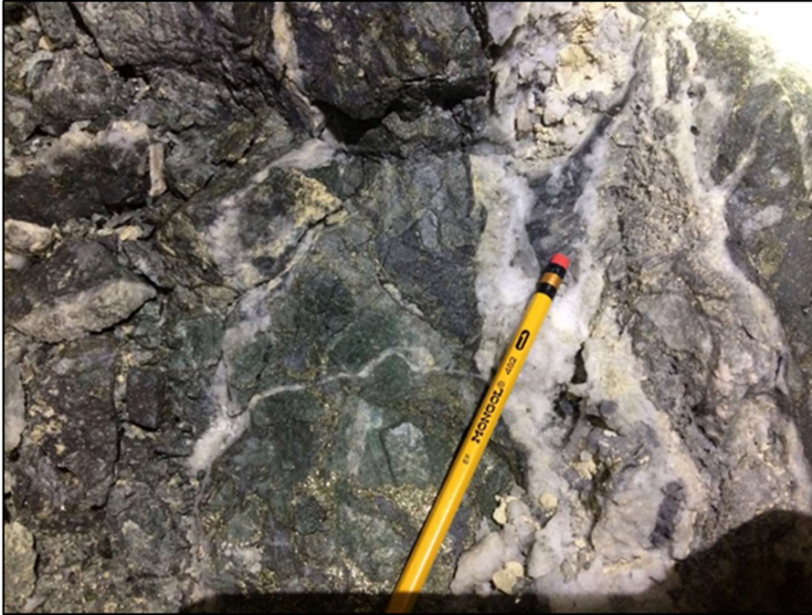
13.1.1.9. Carbonate+quartz vein breccia with py+cpy disseminations and patches exposed underground at heading Level 560 SDNS ODE 102S position.
