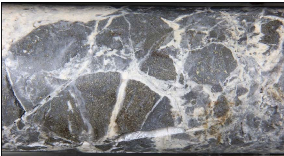
Figure 13.2.1.3: (Cover) ASA-590-004 Intercept – multi-phase breccia with angular to sub-angular sulfide-rich clasts and quartz-calcite-rhodochrosite veins
