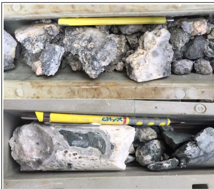
Figure 13.2.1.6: MST-560-004 Intercept at 117.4-117.7m – quartz-carbonate vein breccia with carbonate veins displaying colloform-crustiform banding
