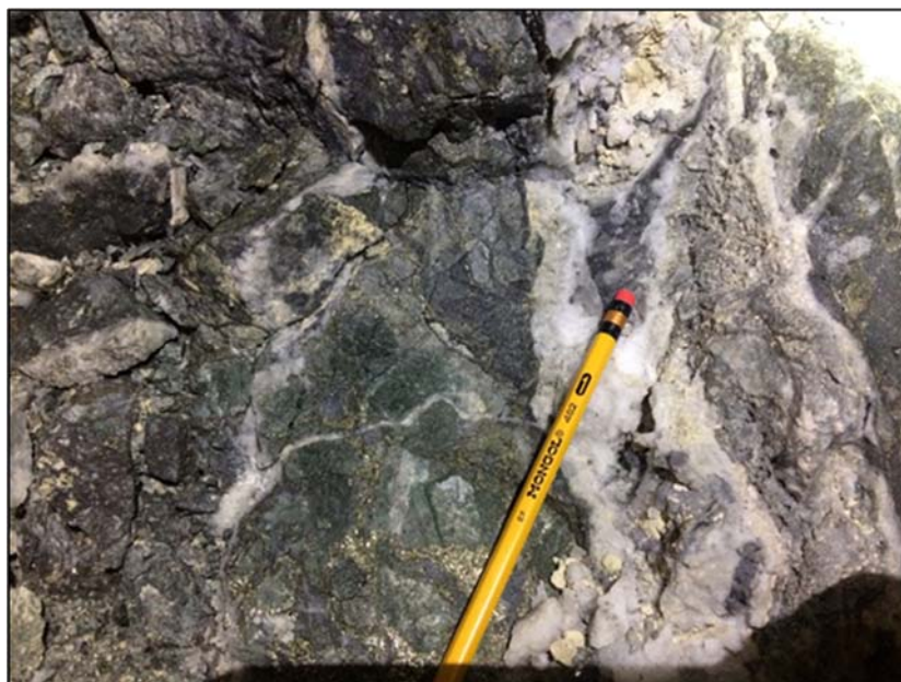
Figure 13.2.1.9: L560 SDNS ODE 102S Drive Exposure – carbonate+quartz vein breccia with pyrite+chalcopryite disseminations and patches
