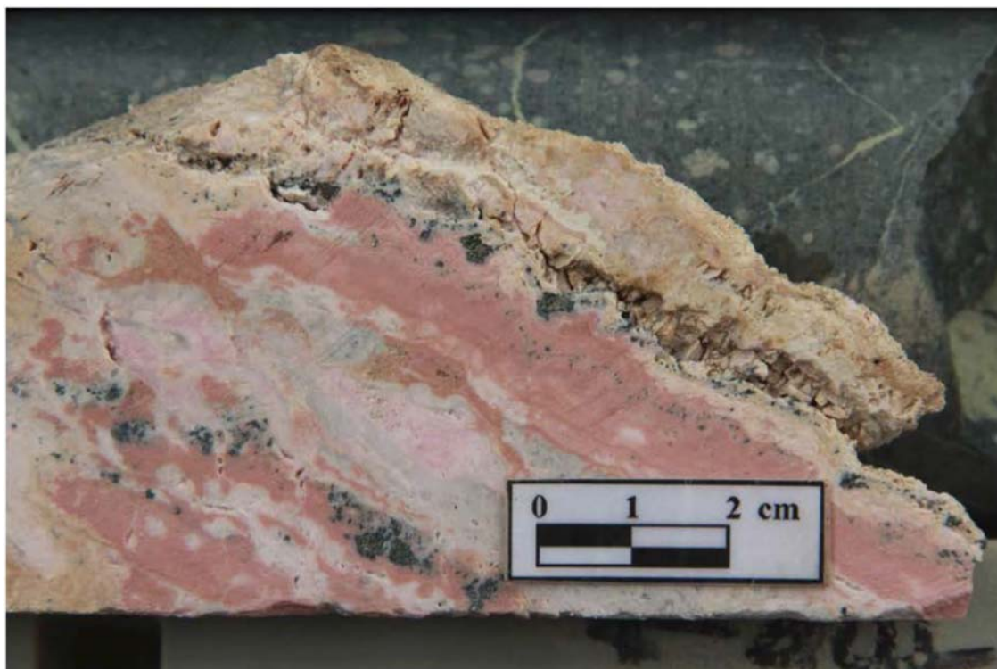
Figure 13.2.1.2: ASA-785-012 Intercept at 330.7m – crustiform-colloform banded quartz+rhodonite+rhodochrosite+sulfide vein and late stage vuggy carbonate veins with bladed texture
