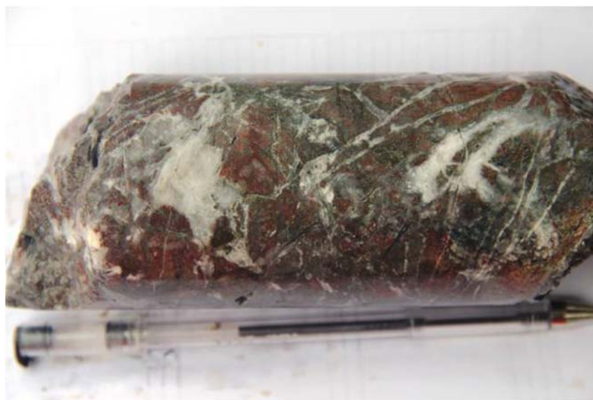
Figure 13.2.3.2: DNC-530-104 Intercept at 85.4m – monomictic crackle breccia characterized by angular garnet skarn clasts set in vuggy, drussy quartz+calcite vein
