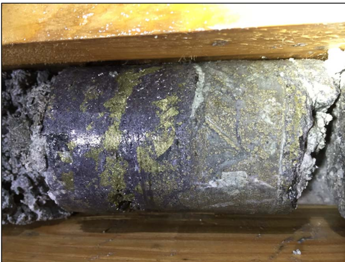
Figure 13.2.1.4: Massive Sulfide (galena+pyrite+chalcopyrite) Vein Breccia Intercept in MST-590-008
