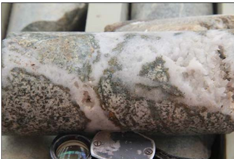
Figure 13.2.1.8: ASA-590-020 Intercept at 56.8-57.8m – vuggy quartz+pyrite+chalcopryite vein with sulfides along vein selvages
