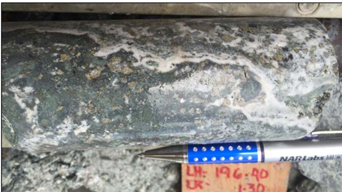
Figure 13.2.1.1: MST-590-005 Intercept at 194.1-195.1m – as part of the Don Calixto vein characterized by multiphase base metal-carbonate mineralization
