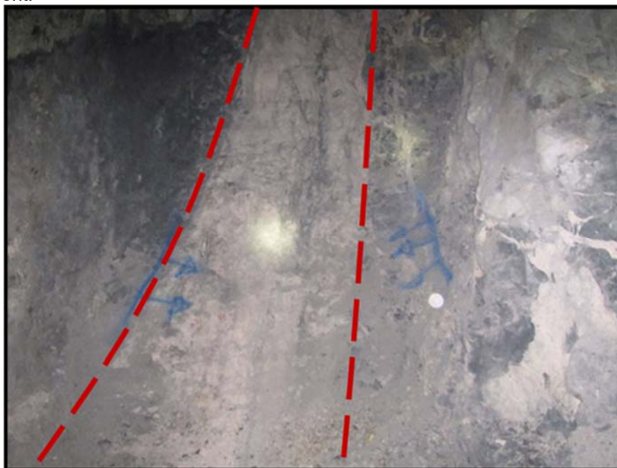
Figure 13.3.1: L590 SDN ODE MV 134S Drive Exposure – 1.2m wide carbonate+base metal sulfide vein composed of carbonates, galena-sphalerite stringers/lenses with minor rhodochrosite and disseminated sulfides (pyrite+chalcopyrite)
