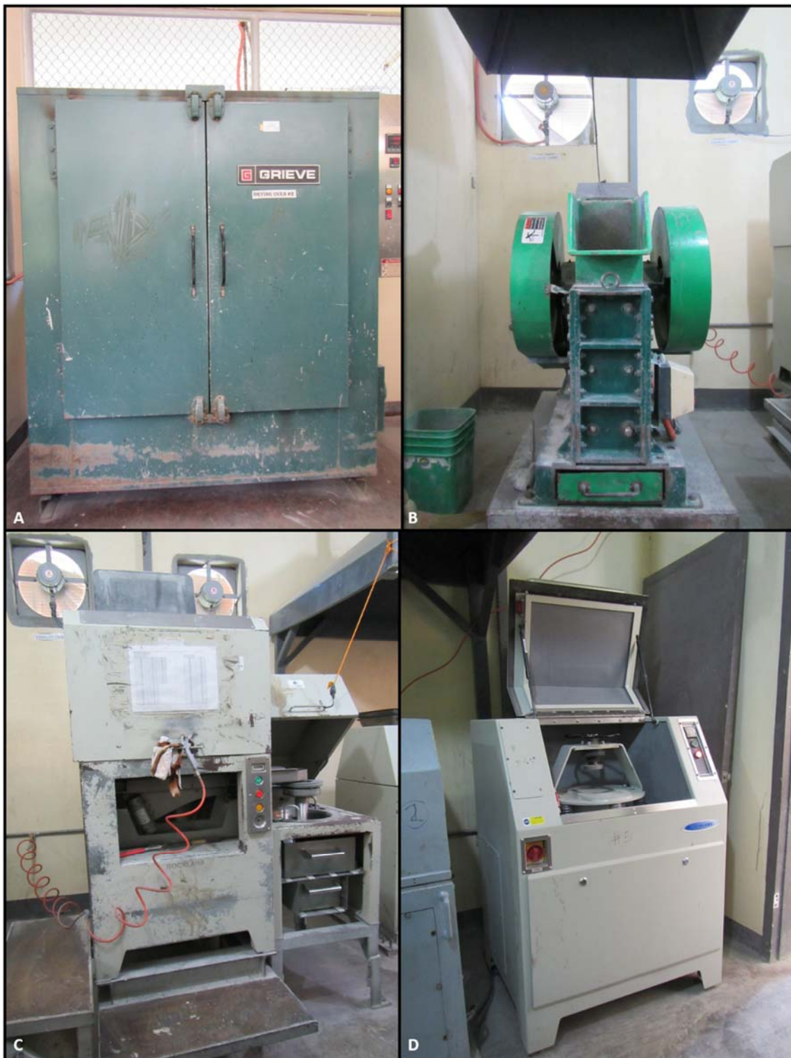
Figure 14.7.2.1.1: Sample Preparation Equipment – (A) Drying Oven (B) Jaw Crusher (C) Boyd Crusher (D) Pulverizer
