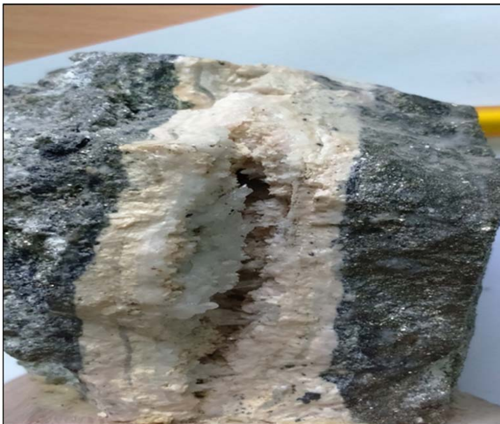
Figure 13.2.1.14: Level 635 SDN ODE Hand Specimen – drusy, vuggy quartz+carbonates in massive sulfide (pyrite-chalcopyrite-galena) vein
