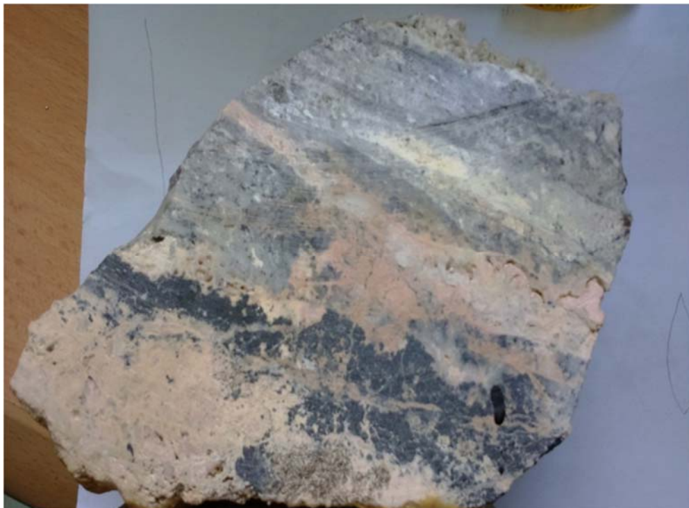
Figure 13.2.1.13: Level 590 SDNS ODW Hand Specimen – quartz-carbonate-galena crustiform-colloform bands with incorporated silicified diorite clasts with relict feldspar laths and disseminated cpy-py
