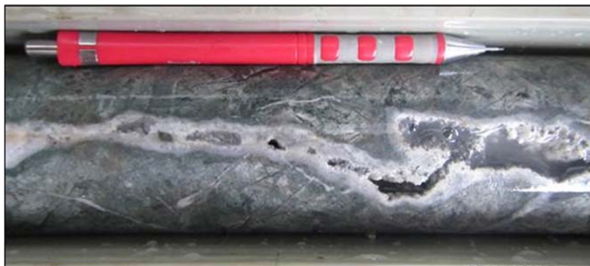
Figure 13.2.1.7: ASA-545-003 Intercept at 116.9-117.1m – vuggy quartz+carbonate vein
