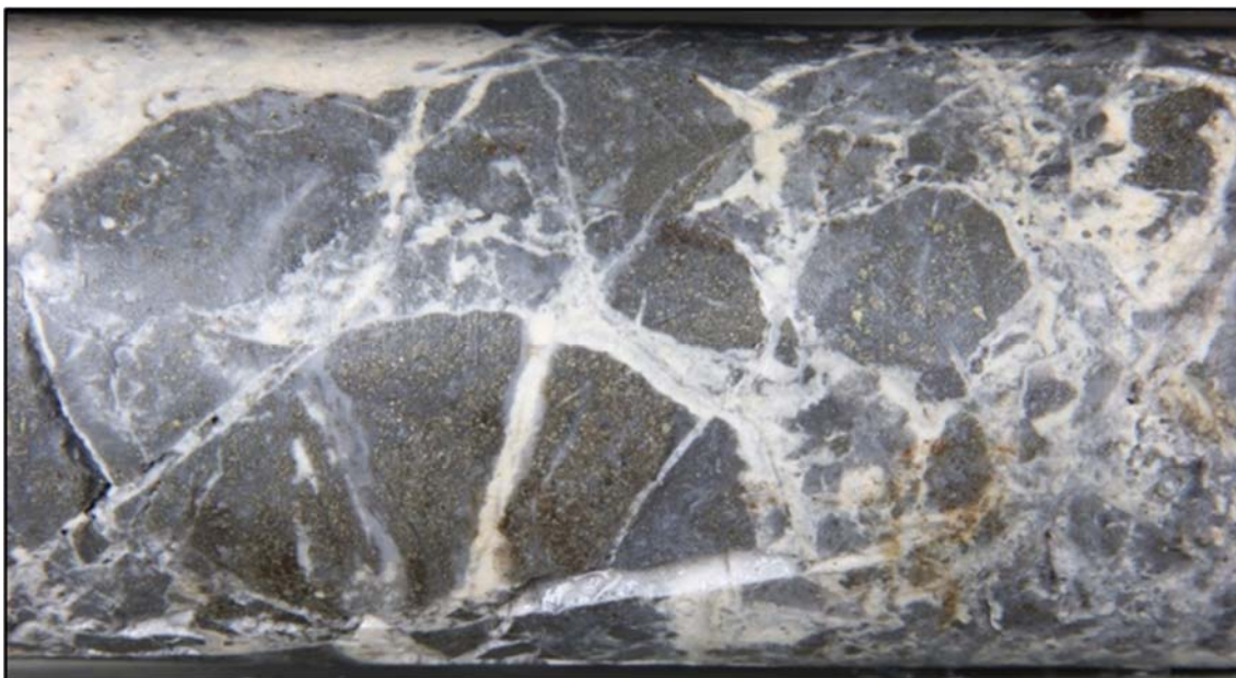
Figure 13.2.1.3: ASA-590-004 Intercept – multi-phase breccia with angular to sub-angular sulfide-rich clasts and quartz-calcite-rhodochrosite veins
