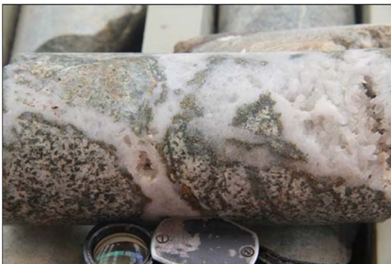
Figure 13.2.1.8: (Cover) ASA-590-020 Intercept at 56.8-57.8m – vuggy quartz+pyrite+chalcopryite vein with sulfides along vein selvages
