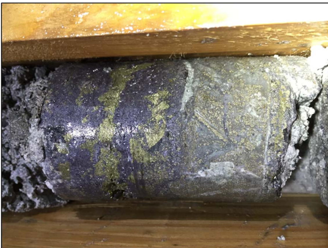
Figure 13.2.1.4: Massive Sulfide (galena+pyrite+chalcopryite) Vein Breccia Intercept in MST-590-008
