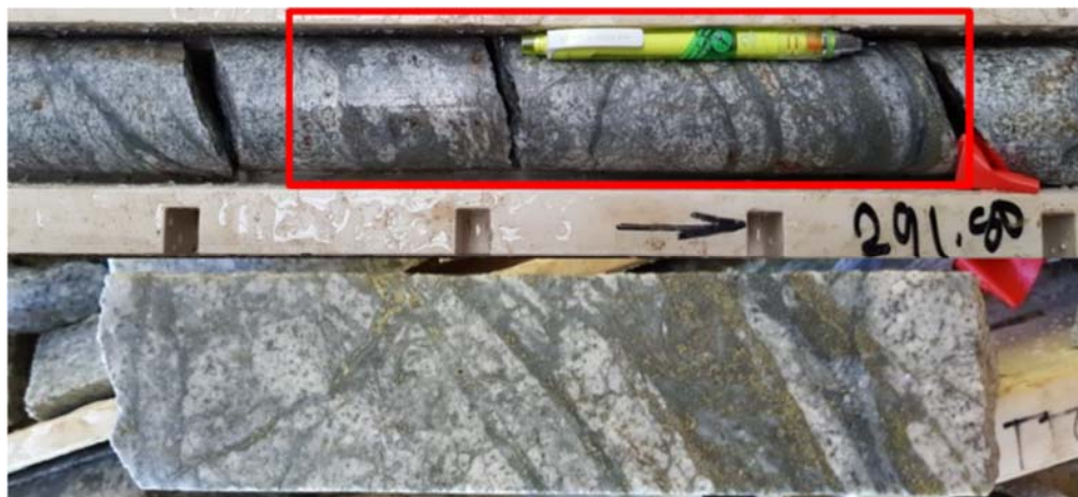
Figure 13.2.1.15: SDN2-605-002 Intercept at 297.8m – wallrock vein breccia with argillic-silicified diorite clasts in a quartz+sulfide matrix
