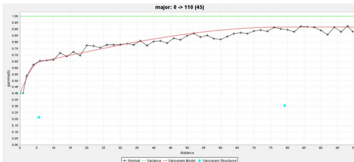
Figure 15.4.1: Experimental Variogram and Fitted Spherical Model for Don Joaquin MV 110 degrees
