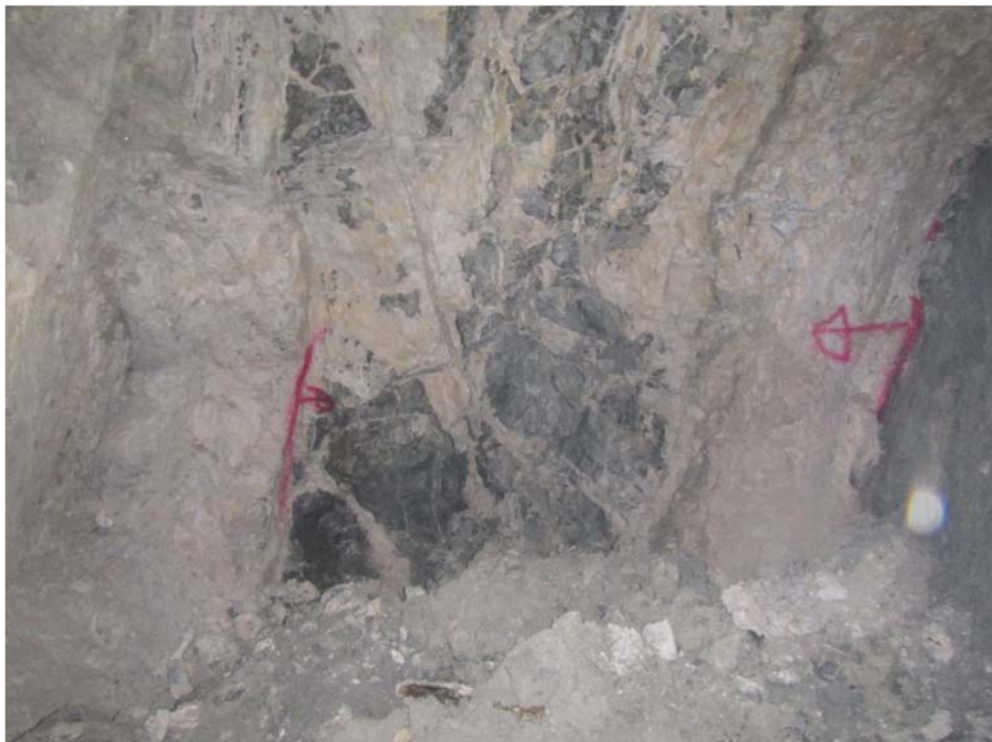
Figure 13.3.3: L756 SDY ODE 142S Drive Exposure – 3.5m wide sulfide-quartz breccia with late carbonates; sulfides are comprised primarily of pyrite and chalcopyrite with minor galena and sphalerite
