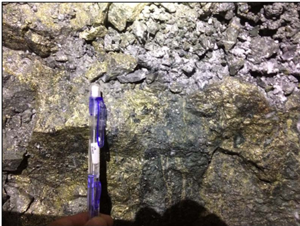
Figure 13.2.1.10: L490 BNZ ODE Drive Exposure – high Au grade massive sulfide (pyrite-chalcopyrite) vein hosted by propylitic-altered andesite
