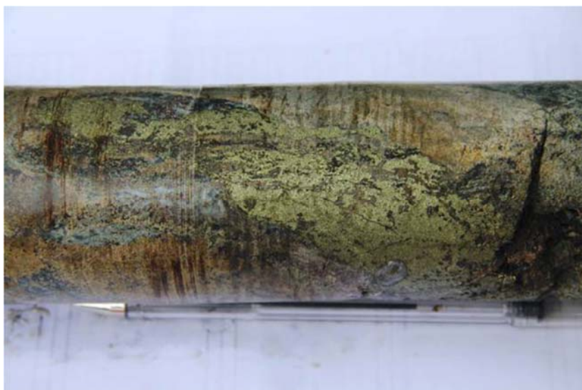
Figure 13.2.3.3: DNC-530-104 intercept at 86.4m – reddish brown garnet skarn with semi-massive chalcopyrite
