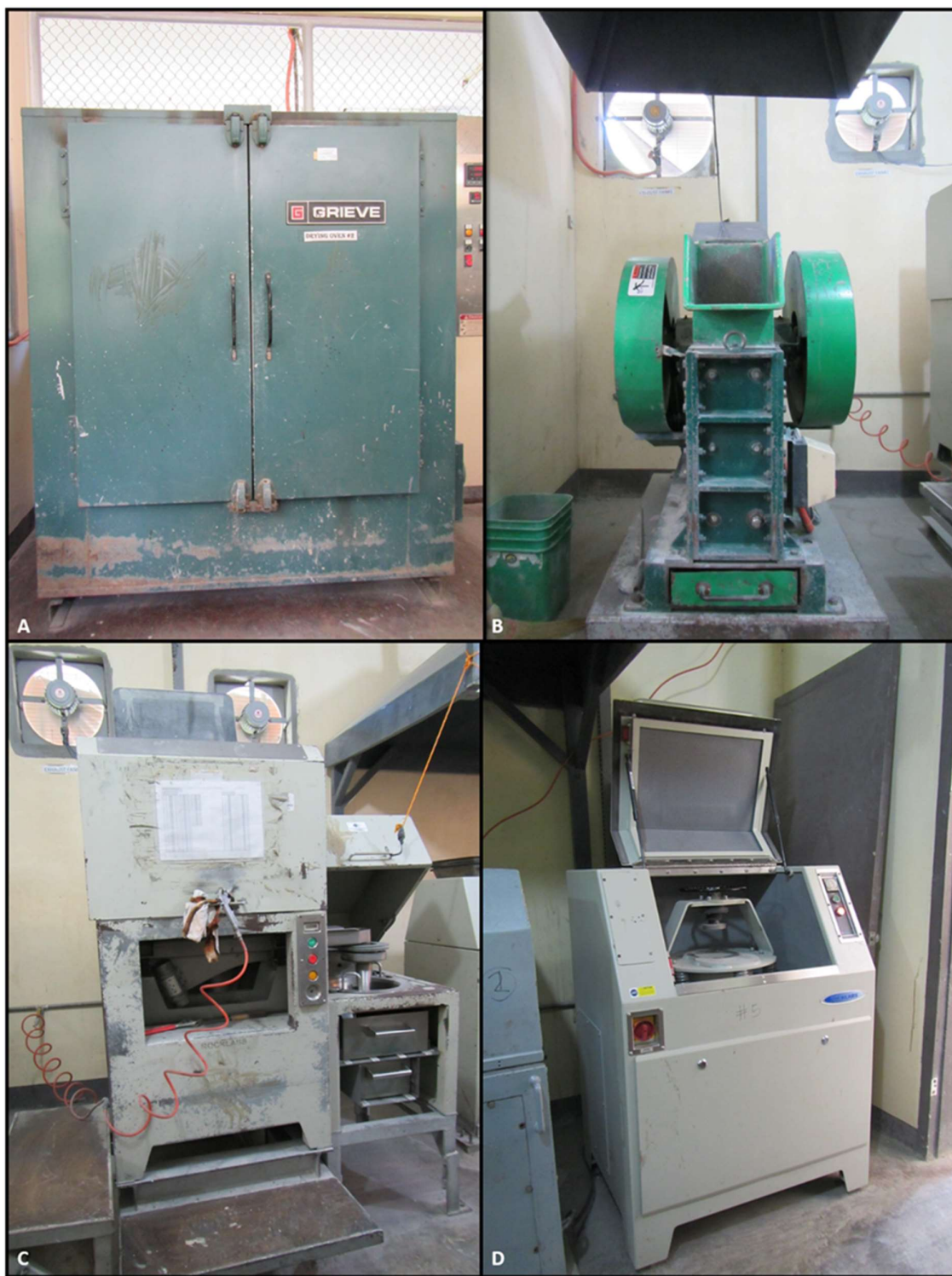
Figure 14.6.2.1.1: Sample Preparation Equipment: (A) Drying Oven (B) Jaw Crusher (C) Boyd Crusher (D) Pulverizer
