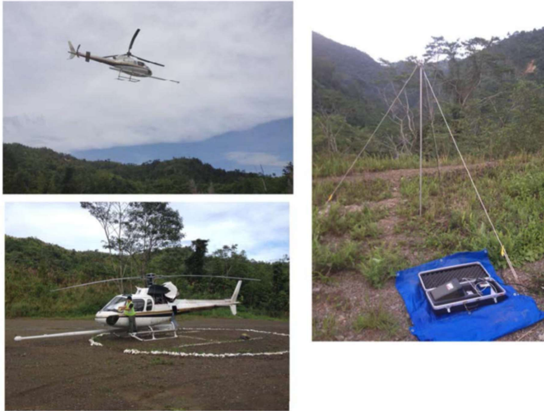
Figure 14.5.5.1.1 Thomson Aviation survey aircraft and base station used for diurnal field monitoring.
